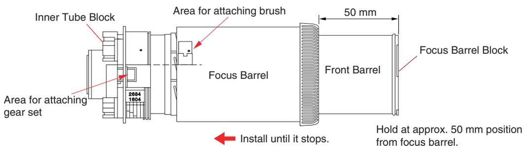
4. Hold the focus barrel block and turn the inner tube block to the position of figure in the direction of the arrow. (The turning is approx. 260 degree, so that the projection goes over about 5 mm from the area for attaching brush.)
