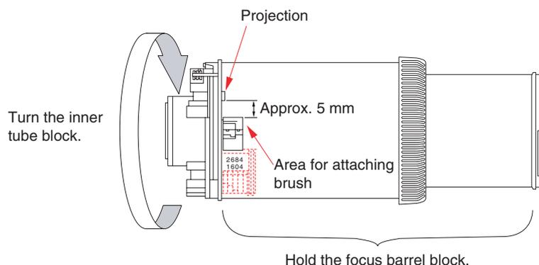
5. Insert the front barrel to the inner tube block until it stops.
