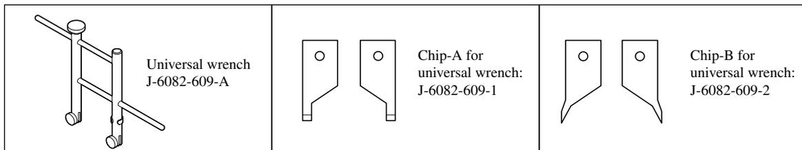
Attach the chip-A or chip-B to the universal wrench.
