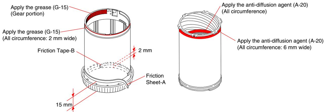
4. Insert the front barrel to the focus barrel as shown in the figure.
