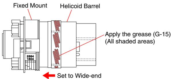
3. Fit the focus barrel to the inner tube block, and install the focus barrel to the inner tube block until it stops at the inner tube block.
