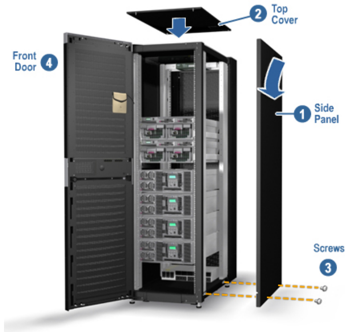
Figure 2–10 Replacing the Side Panel
