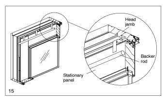
Use a stiff putty knife to bend the head jamb brackets into place. See illustration 16. Fasten the head jamb bracket to the head jamb with four #8x1" flat head screws placed at a 45° angle. See illustration 16.
