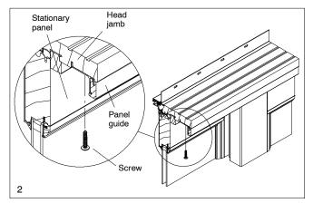
Open operating panel and allow door panel to tilt inward, lift panel guide off of top stile. Save for reuse later. Lift upward on panel until rollers are disengaged from the sill and remove from frame. See illustration 3.
