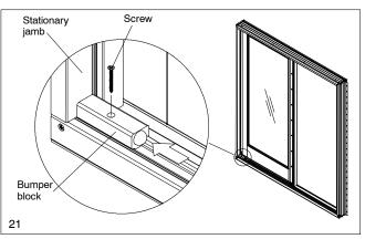
13. Set the operator panel onto the track. Reinstall the operator panel guide and top bumper block. See illustration 22.
