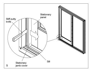
7. Remove the condensation cover from the sill by using a stiff putty knife. *Note: The condensation cover is secured to the sill by a vinyl barb.* See illustration 6.
