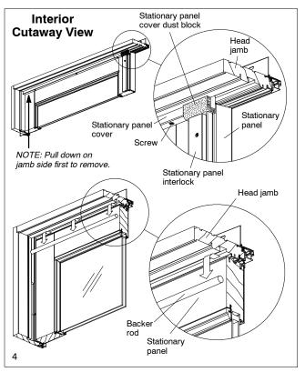
6. Starting at the top, remove the stationary jamb cover using a stiff putty knife. *Note: The cover is attached to the jamb by a vinyl barb.* See illustration 5.
