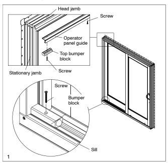
3. Slide operating panel to the stationary jamb side of the frame. Remove exposed screws securing the panel guide to the head jamb. Next, move the operating panel to the closed position and remove remaining screws securing the panel guide to the head jamb. See illustration 2.
