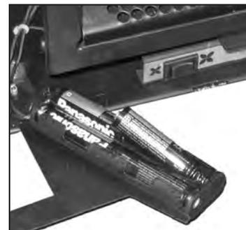
Figure 12: Battery Clip on Bracket.
