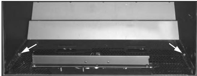
Figure 15: Screws Holding Burner Tray in Place.
