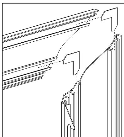
**Figure 59: Corner brackets being Installed into Trim.**
