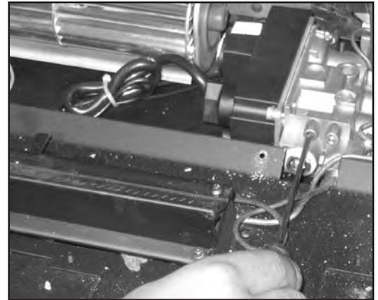
**Figure 55: Opening Inlet Pressure Tap on Valve.**
