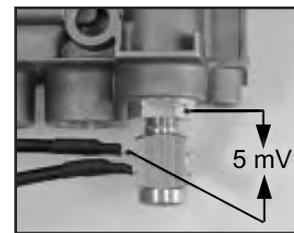
**Figure 80: Voltage Across Valve's Spade Connector.**
