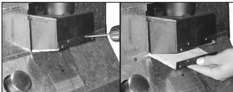
**Figure 34: Remove Flue Slider Plate & Gasket.**
