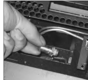
**Figure 22: Orifice Replacement.**
