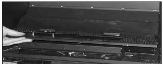
Figure 16: Removing Burner Tray.
