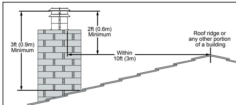
**Figure 37: Roof Clearances.**
