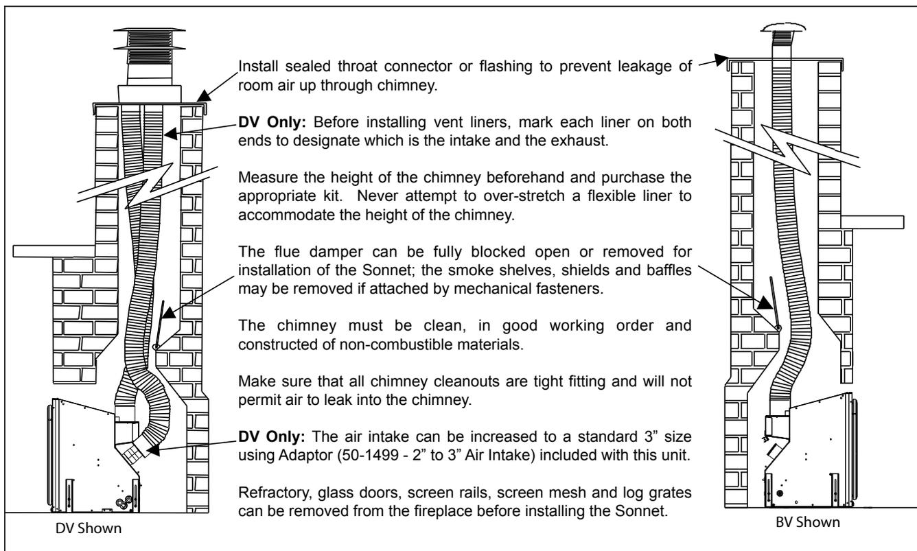
**Figure 38: Installation of Sonnet DV and BV.**
