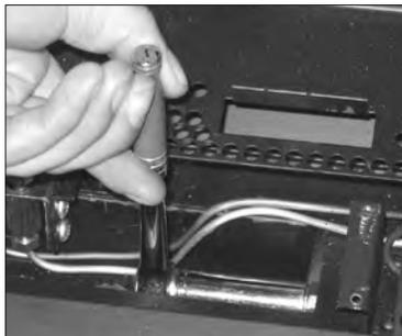
**Figure 21: Orifice Removal.**
