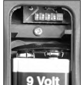
Figure 13: DIP Switch in Remote Handset Battery Compartment.
