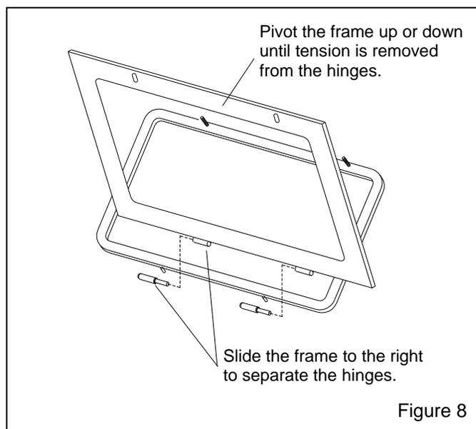
**7.5.5** Replace the frame in reverse order. Align the top bolt holes with the bolts; slide the frame as necessary.
