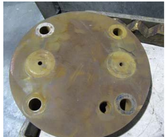
LEFT – Typical housing wearing in a crude oil application. Note : Although rotor bores may look in relatively good condition, running clearances between rotor OD’s and housing bores could be well outside application-dependent values. For example, there may be pump efficiency limits or maximum allowable vibration levels. Maintenance cycles and wear may also vary from location to location, as well as differences in fluid particulate content/size and fluid viscosity. Good record keeping is vital in determining changes and will provide a baseline when troubleshooting is required. RIGHT – Typical thrust plate wear in crude oil applications.
