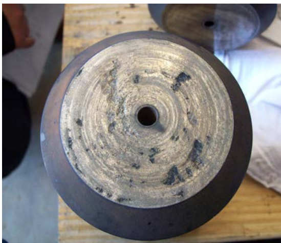
Idler cup and shoe normal wear in an application with high sand content. Bottom of cup (left) shows some damage where metal has been “picked out”- possibly cavitation.
