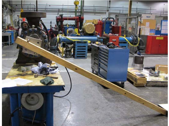
Above photos show proper way to lock shaft in position to break lock-nut free on shaft.
