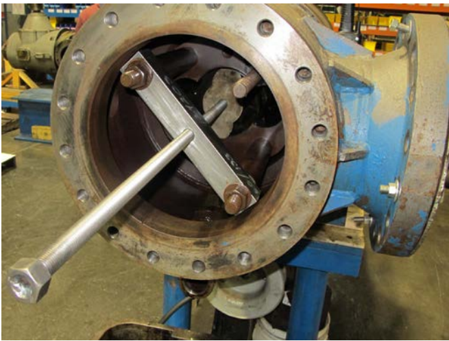
LEFT – Pressing power rotor out of inboard cover. If shaft is to be reused, ensure a blank is placed between power rotor removal strongback (S626MN) and outboard end of power rotor. RIGHT – Mechanical seal/bearing installation.
