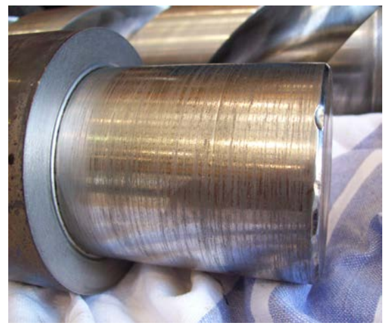
Idler cup and shoe normal wear in an application with high sand content. Bottom of cup (left) shows some damage where metal has been “picked out”- possibly cavitation.
