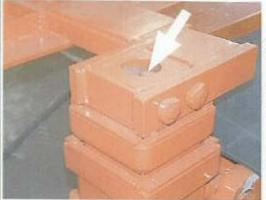
The driller canopy support post assembly is made up of three nested square tubes, supported by a hydraulic cylinder. A bolt, located at the top of the housing assembly, provides the connection between the tubing and hydraulic cylinder.
