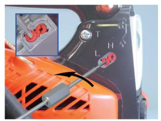
Tools Required: Small screwdriver with 2.5 mm blade, electronic tachometer P/N 897801-33330, limiter cap removal tool with 2.5 mm left-hand thread P/N 91019. Parts Required: (2) limiter caps P/N P003-000010.
