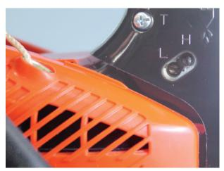
5. Turn L and H mixture needle clockwise until lightly seated, and then turn both mixture needles anticlockwise following turns.
