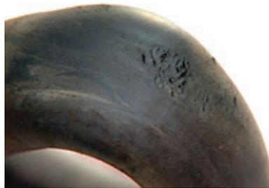
Cracked hose. This hose has cracked and will soon start to leak.
