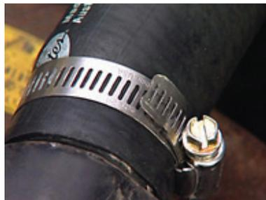
Gear or worm-type clamp. Adjust with a screwdriver.
