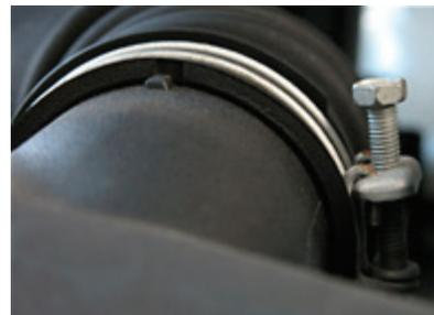
Banded or screw-type clamp. Also adjusted with a screwdriver.
