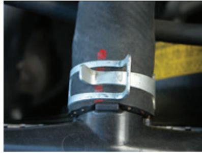
Wire clamp. This spring clamp is not adjustable and is fitted and removed with special hose clamp pliers, which have grooved jaws.
