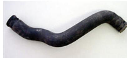
Hardened hose. This hose has become brittle and will break and leak.
