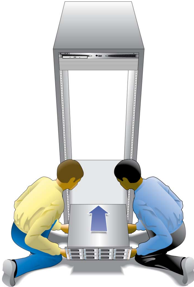
FIGURE 2-12 Positioning the Controller Tray in the Cabinet
