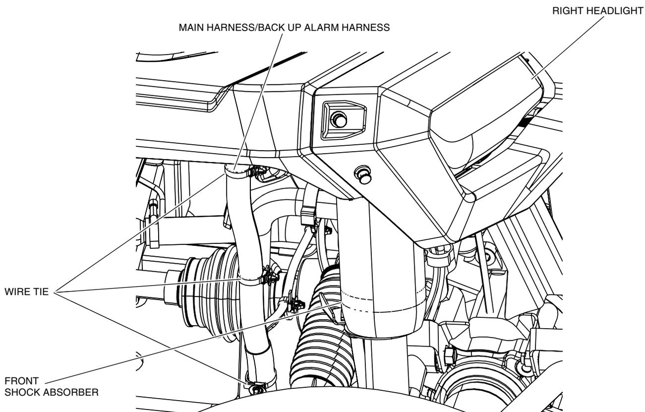
6. Locate the DLC (4P Red) connector and remove the dummy cap. Be sure to leave the black tape around the connector body (harness side).
