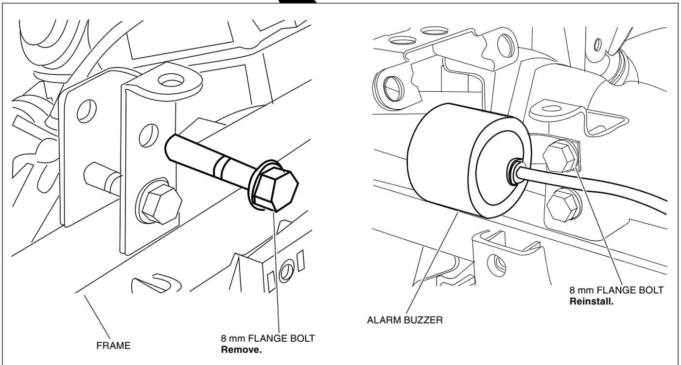
9. Connect the back up alarm buzzer connector to the back up alarm harness.
