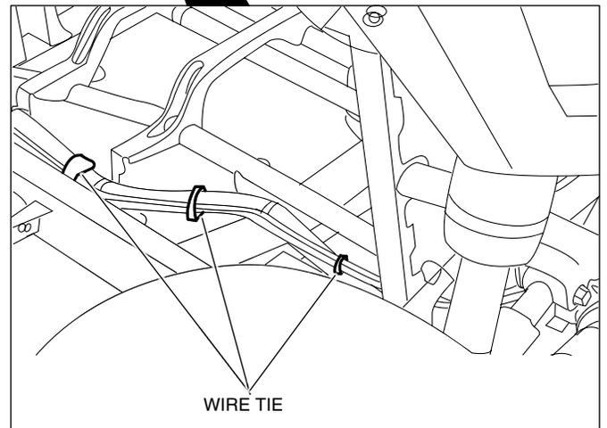
5. Follow the main harness going up. Secure the back up alarm harness to the main harness with wire ties along the front right side of the vehicle as shown.
