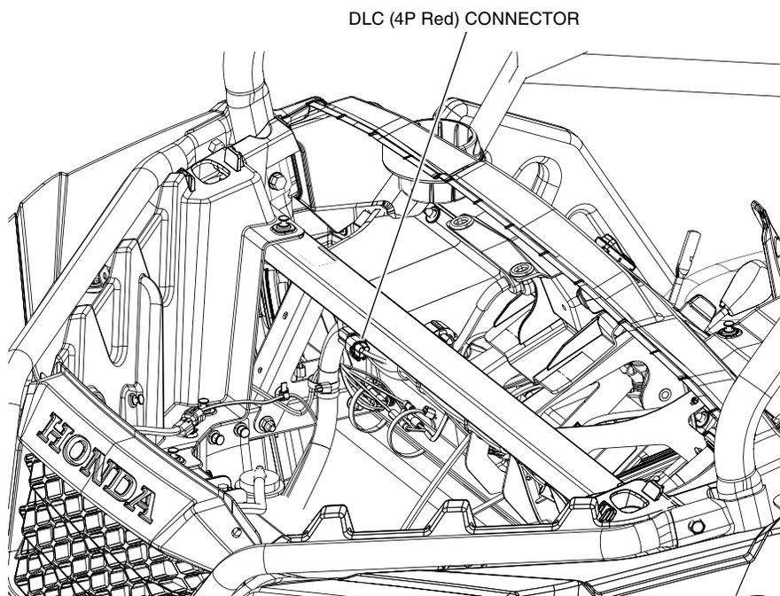
7. Connect the accessory sub-harness to the DLC (4P Red) connector.
