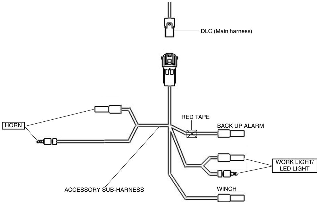
8. Install the back up alarm buzzer to the location shown:
