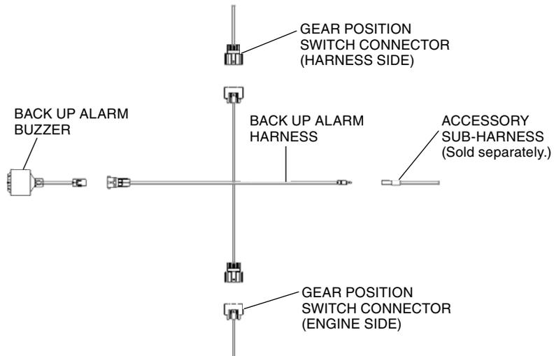
4. Follow the main harness down. Secure the back up alarm harness to the main harness with wire ties near the back of the engine, under the passenger seat as shown.
