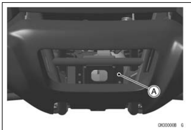
A. Winch-installing position
