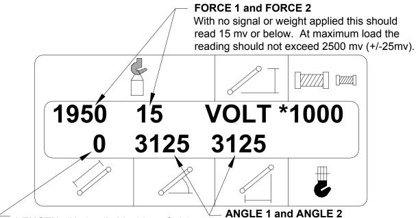
**LENGTH** (Hydraulic Machines Only) reading should be 0 with no sensor installed.
