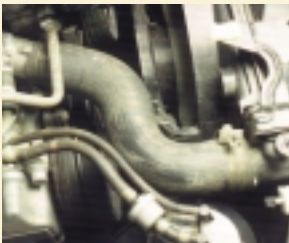
Cooling System Hoses
