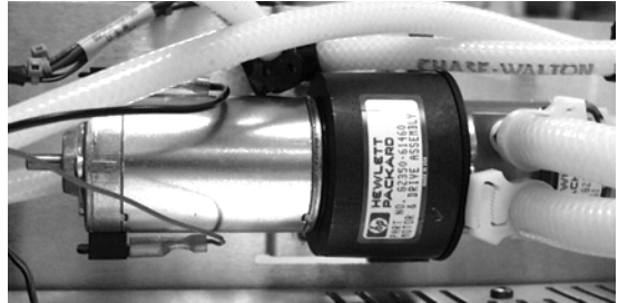
Type 2 – Bracket on side of water drawer AED serial number between US01000166 and US03000388
