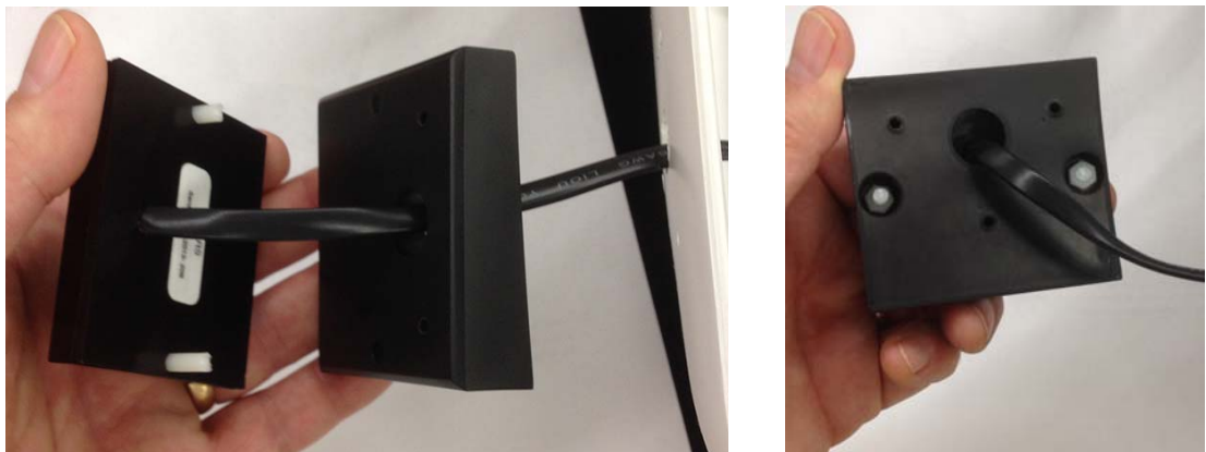
Figure 2-13 Assemble receiver and receiver mount
