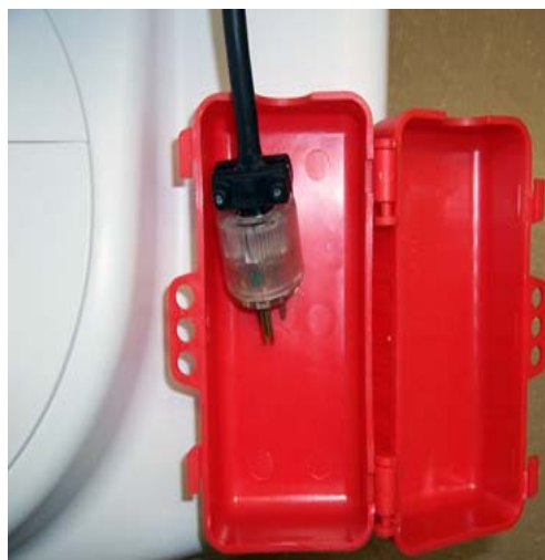
Figure 1-4 AC power plug with locking device applied
