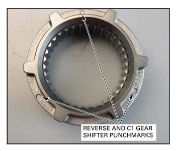
When installing the shifter, position it with the punch-marked side facing the C1 gear.
