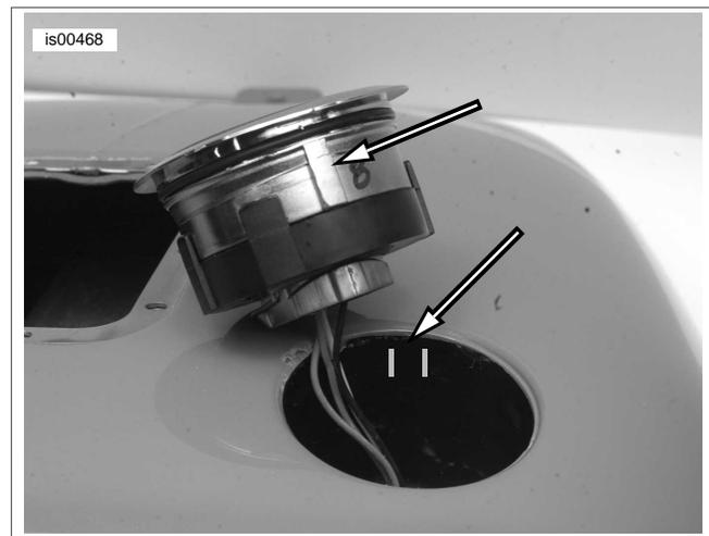
**Figure 6. Align Wide Tab with Rear Tabs in Fuel Tank Cup**
