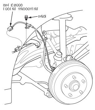
4. Pull the EVAP hose off the drain joint, then remove and discard the drain joint.
