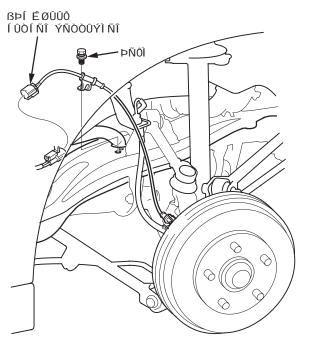
3. Pull the EVAP hose off the drain joint, then remove and discard the drain joint.
