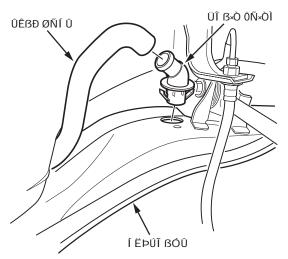
5. Disconnect the EVAP canister lines from the canister, then blow compressed air through the lines to clear them of any water or ice.
