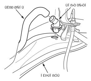
4. Remove any Hondabond material from the drain joint area on the subframe.
