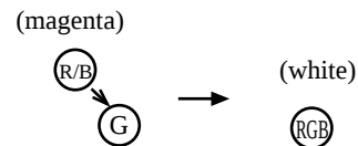
Align the G beam with the R/B beam Fig. 1-3
