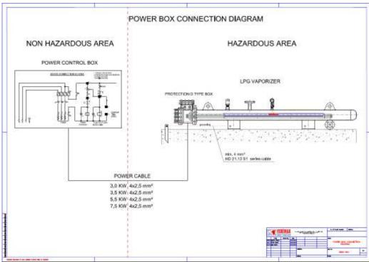
1x 4 mm<sup>2</sup> grounding cables must be used for grounding vaporizer and grounding value must be lower than 3 ohm. This grounding cable can be connected to M10 bolt connected to the vaporizer foot.
