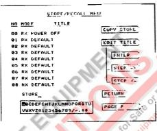
26 non-volatile stores are provided, each capable of . ataining indefinitely a complete front panel set-up, with instant recall whenever required. Each store may be allocated an alphanumeric title of up to 20 characters to remember its contents. One additional storage location (00) provides power fail back-up so that the last group of front panel settings is restored after an AC power or battery supply failure. A facility is provided to lock the stores to prevent accidental erasure.
