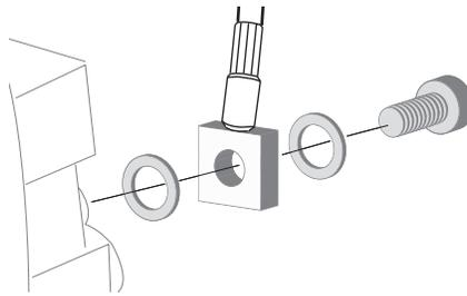
**HINT:** Install with new copper washers as indicated above, making sure brake line will not contact tire.
