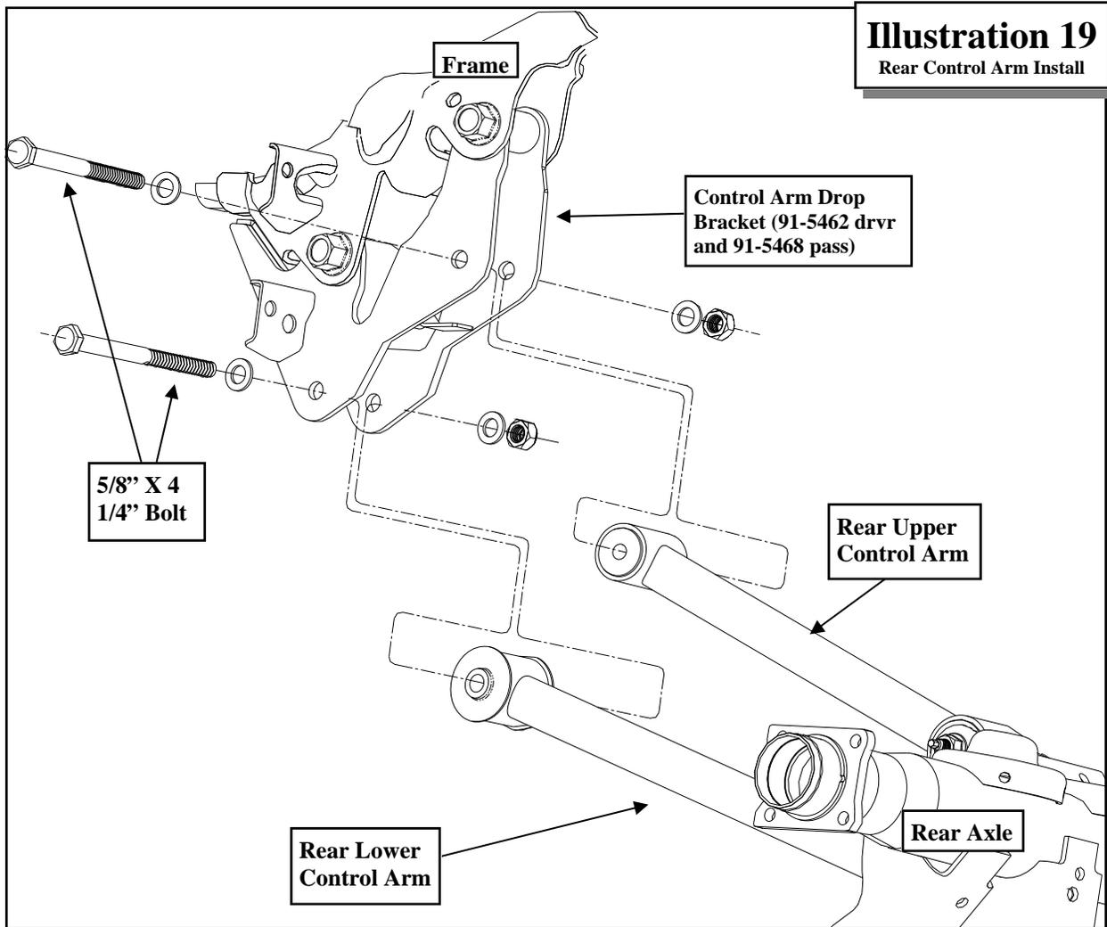
moved OE control arm bolts. Secure the front of the bracket to the frame using the supplied nut plate (90-5472) and 1/2" X 1 1/2" bolt and hardware. See ILLUSTRATION 18.
