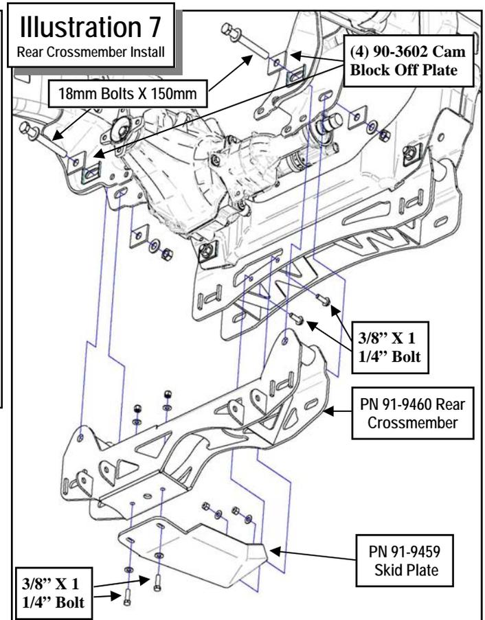
cam block off plate (**90-3602**). Leave hardware loose at this time. See ILLUSTRATION 6.
