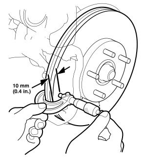
3. Replace the front brake pad set (refer to steps 10 thru 16 on page 19-12 of the 1999-01 3.2TL Service Manual or steps 10 thru 16 on page 19-12 of the 2001-02 3.2CL Service Manual).
