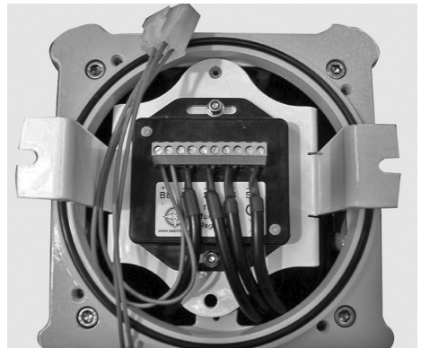
SL10 AMP Regulator shown when correctly fitted
