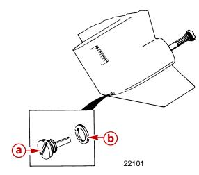
a - Fill/Drain Screwb - Sealing Washer Or O-ring
