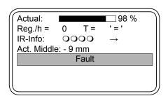
Faults of the systems are displayed in the 5<sup>th</sup> line of the display of the digital control unit DC 761. At the same time the red alarm LED is flashing, and the alarm output is switched on (terminal NK 3501, clamp 32).
