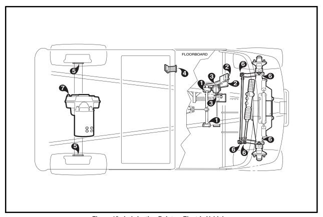
Figure 18 Lubrication Points – Electric Vehicles
