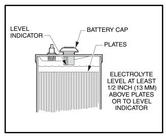
Figure 20 Electric Battery Electrolyte Level
