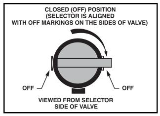
Figure 15 Fuel Shut-off Valve - Closed Position
