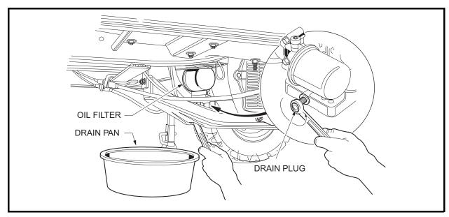
Figure 27 Engine Oil Drain Plug and Pan
