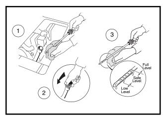
Figure 26 Engine Oil Level Check
