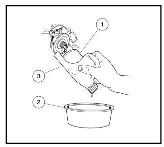
Figure 28 Remove Engine Oil Filter
