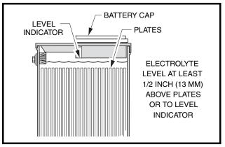
Figure 25 Gasoline Battery Electrolyte Level
