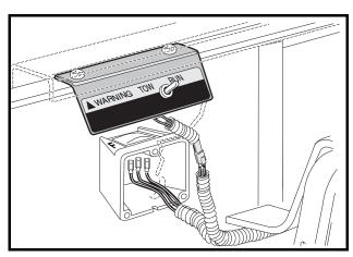
Figure 10 Tow/Run Switch
