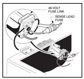
Figure 23 Receptacle Fuse Link
