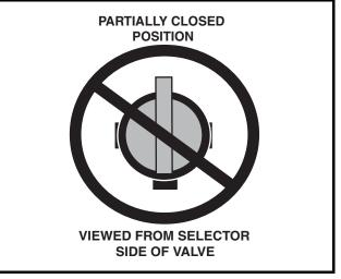
Figure 17 Fuel Shut-off Valve – Partially Closed Position
