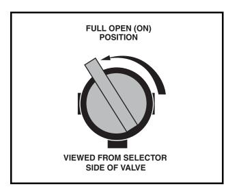
Figure 16 Fuel Shut-off Valve – Open Position
