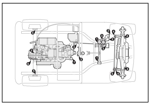
Figure 19 Lubrication Points – Gasoline Vehicles
