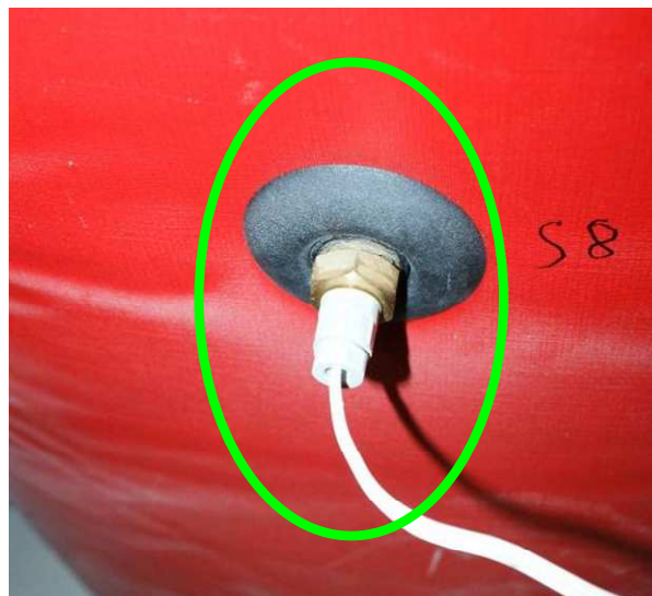
Figure 12: Temperature sensors fixed correctly [[3]]
