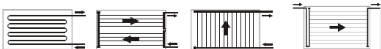
Figure 3: Collectors with good emptying behaviour [[2]]
