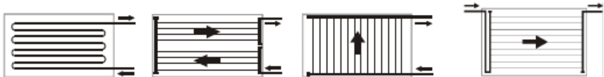
Figure 11: Collectors with good emptying behaviour [[2]]
