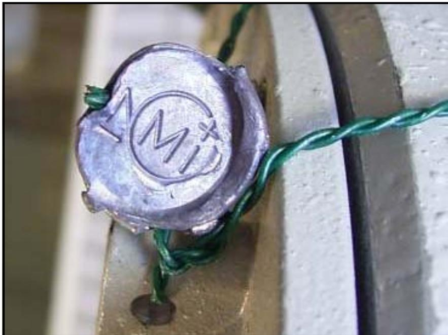
**Figure 42: NMI Lead Seal - Typical**
