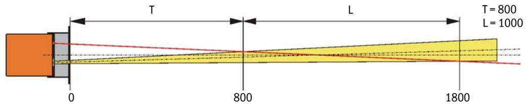
Immersion depth and measuring volume length can be changed easily onsite (→ p. 34, §4.1.1)
