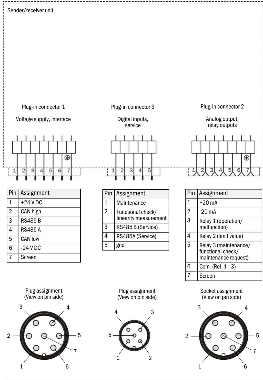
**NOTICE:** Only one RS485 interface may be connected at any one time (either on plug-in connector 1 or on plug-in connector 3). Otherwise, communication errors will occur.
