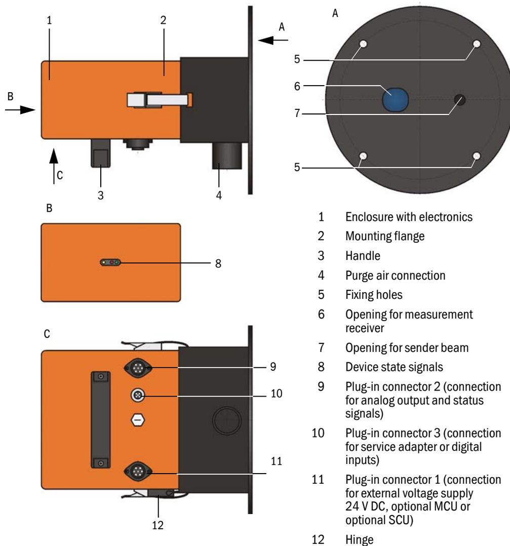
The current device state (operation/malfunction, maintenance/maintenance request) is signaled on the rear side of the enclosure (green = operation, red = malfunction, yellow = maintenance).
