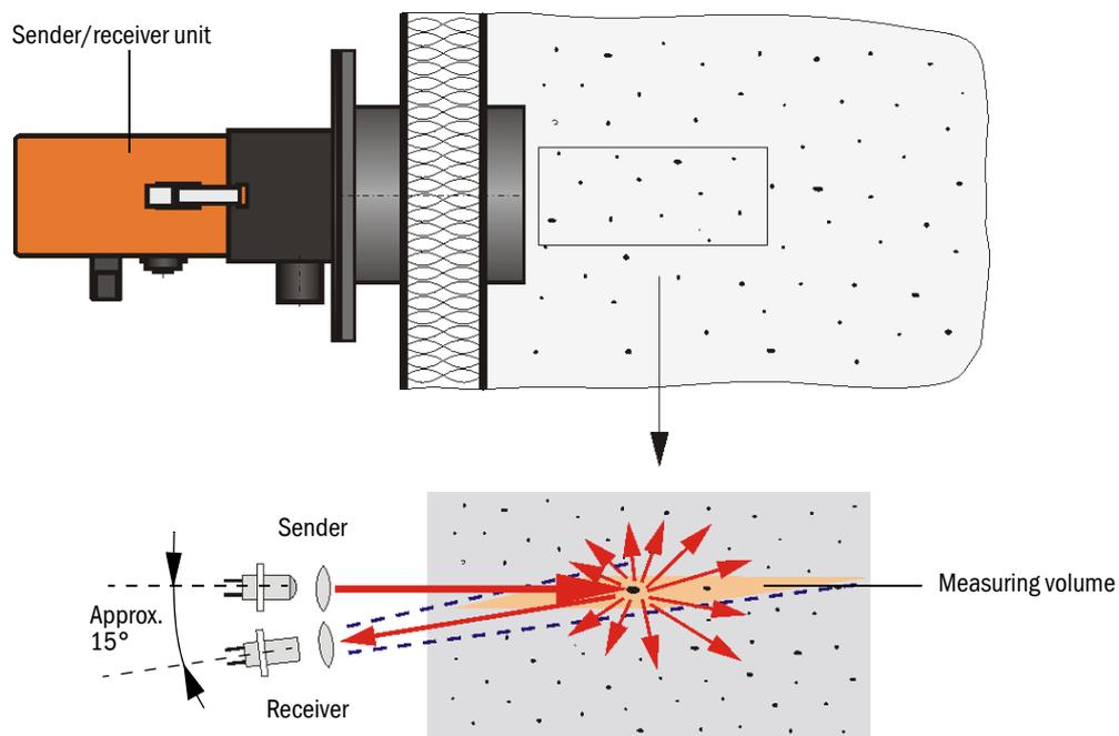
The incline of the control receiver can be modified for differing internal duct diameters. A small light trap may be required in certain cases for very narrow internal duct diameters (most unfavorable conditions for background light).
