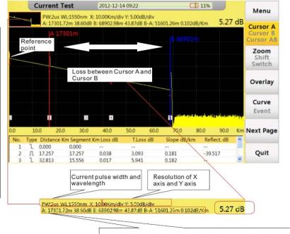
Indicate distance of cursor A and cursor B which relative to the reference point(start event), relative distance(km) and loss(dB) between cursor A and cursor B.
