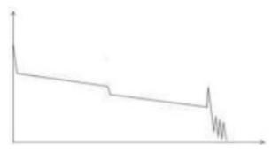
Sometimes, the loss value could be a negative value; it does not means the loss does not exist. It is common phenomenon called pseudo gain, it is by a connection of two fibers with different back scatter coefficient, the scatter coefficient of the back fiber is large than the front one's. In addition, the different refract ratio also can cause the phenomenon. To avoid it, we could test a fiber bi-directionally.
