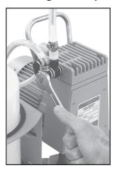
■ Use open-ended wrench w/f 17, remove the screw-in fittings together with the hose from the pump heads.
