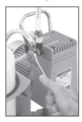
■ Use open-ended wrench to assemble fittings with connection hose to the pump head.
