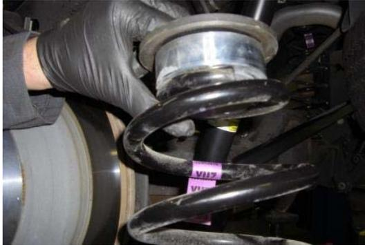
The ReadyLift coil will mount on top of the coil.
