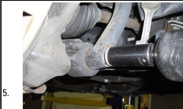
Loosen but do not remove the lower strut mounting nut.
