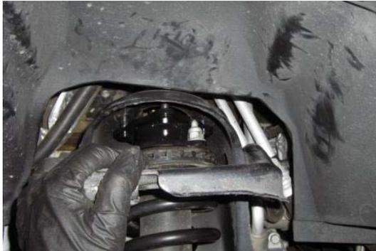
Install the strut into the OEM location. The ReadyLift kit has three mounting studs that locate into the existing holes in the strut tower. Loosely install the upper strut mounting nuts.
