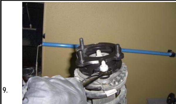
Place the lower strut mount in a vise. Install the ReadyLift strut extension using the factory nuts. Tighten to 42 ft-lbs.
