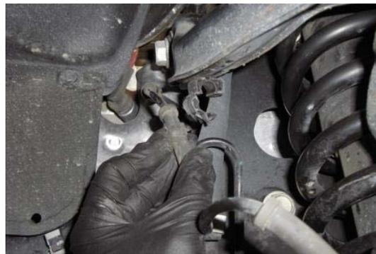
Also disconnect the ABS line from the support bracket on the upper control arm.
