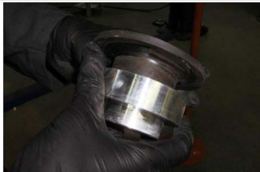
20. Take the isolator and install it into the ReadyLift coil spacer.
