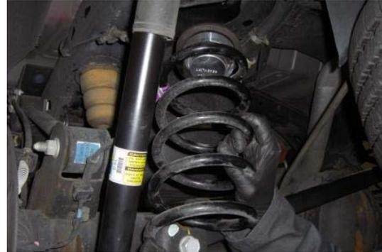
Lower jack enough to reinstall the factory coil with the ReadyLift spacer on top of it.
