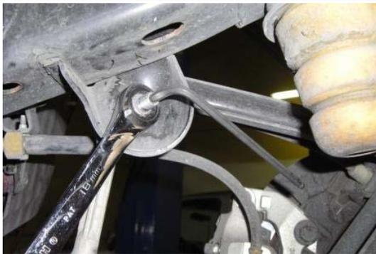
17. Starting in the driver side, unbolt the upper sway bar end link.
