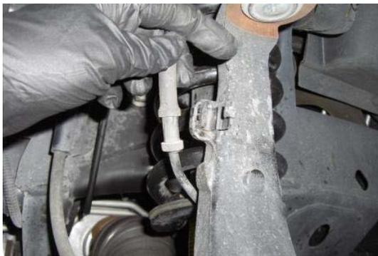
Remove the front wheels. Starting on the driver side, disconnect the ABS line from the support bracket at the knuckle.
