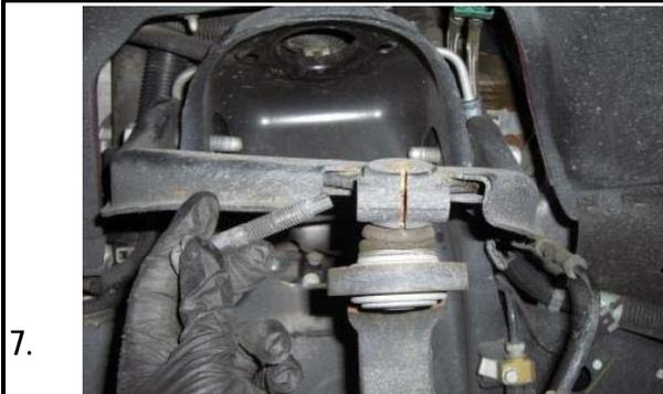
Remove the two upper strut mounting nuts and remove the strut. Support the lower control arm with a jack. Unbolt and remove the upper ball joint retaining bolt.
