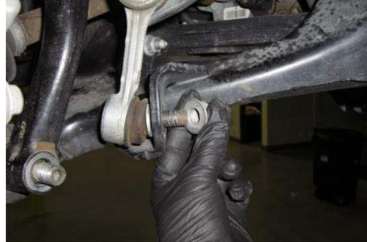
Lower the jack and install the lower strut mount and nut but do not tighten. Tighten the strut arm pinch bolt. Reinstall the lower sway bar end link.
