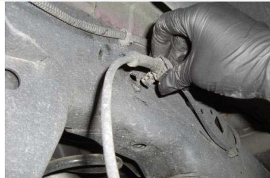
16. Unclip the ABS Line from the frame rail on both sides. Use a jack to support the rear axle.
