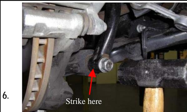
Use a pitman arm puller or similar tool to break the taper. If not available, you can use a hammer to free the taper by striking the lower strut mount while prying on it.
