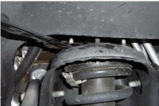
Loosen, but do not remove the two upper strut mounting nuts.
