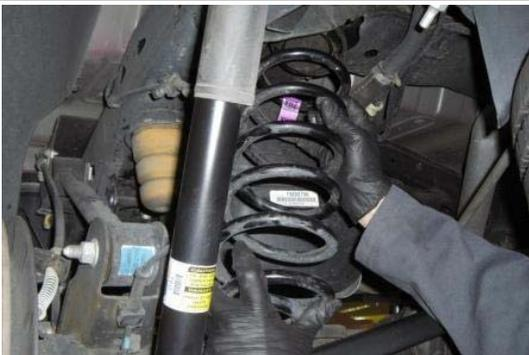
19. Lower the jack enough to remove the coil spring and isolator.
