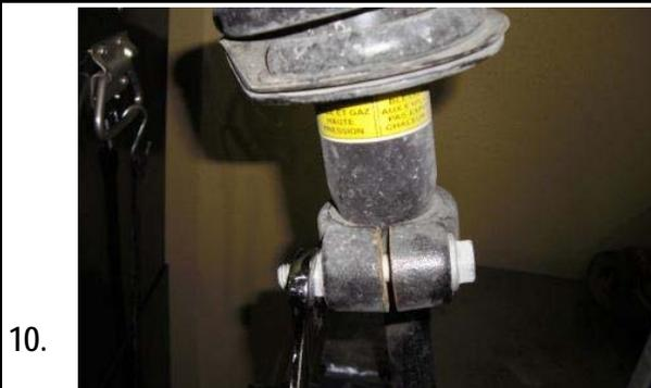
Loosen, but do not remove the strut arm pinch bolt. This allows this strut to rotate around for reinstallation.
