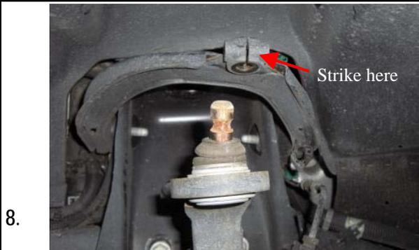
Use a ball joint separator or other appropriate tool to break the ball joint loose from the upper control arm. If tool is unavailable to you, taper can be freed by striking the upper control arm with a hammer. Lower the jack.
