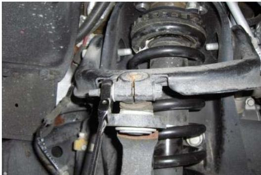
Raise the jack to compress the suspension, Reconnect the upper ball joint to the upper control arm. Insert the retaining bolt and nut, tighten to 42 ft-lbs.
