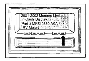
1. With the key in the OFF position, push and hold the "DISP" button.
