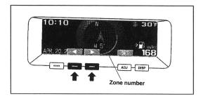
3. Press either the " < ," or " > " function button until the correct zone number appears in the display.
