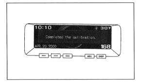
4. After driving in circles, the adjustment completes automatically, and this message displays verifying completion of adjustment.
