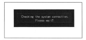
3. As instructed in the display in step 2, turn the ignition key to the ON position to start the system-connection - check.
