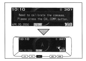
1. If the compass requires manual calibration, the "Need to calibrate the compass" message will appear on the display for about 7-seconds and the direction indicator will blink. Press the CAL COMP function button.
