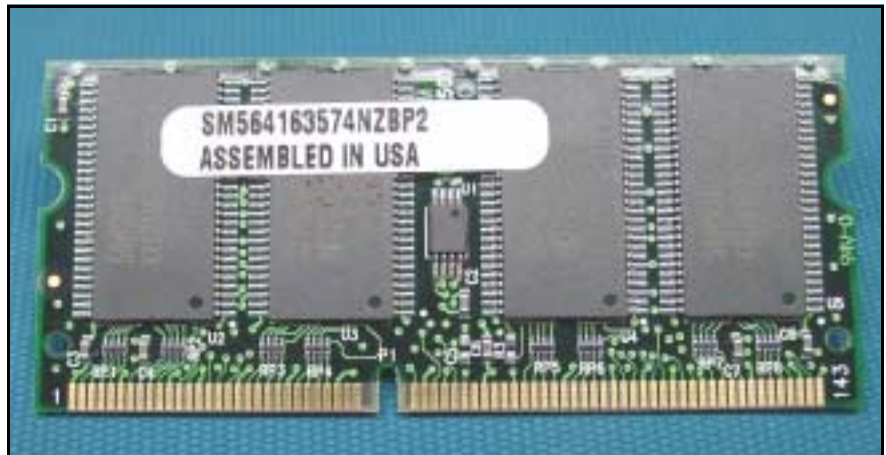
Figure A-2 128M Memory Module
