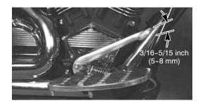
If the brake pedal travels too far before beginning to engage the brake, see the *Victory Service Manual*, or contact an authorized Victory dealer for service.
