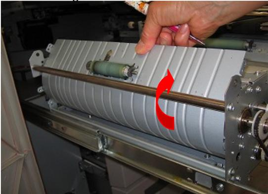
11. Take the roller and its springs out from the guide and fit them in to the new guide plate.
