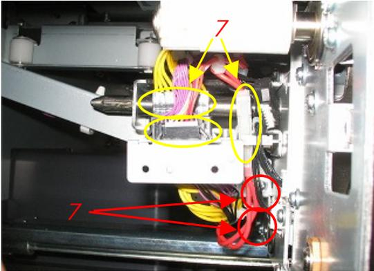
8. Remove the ADU drive board (3 screws, 8 connectors)
