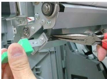
Remove the hook of spring on release lever (Rear spring)
