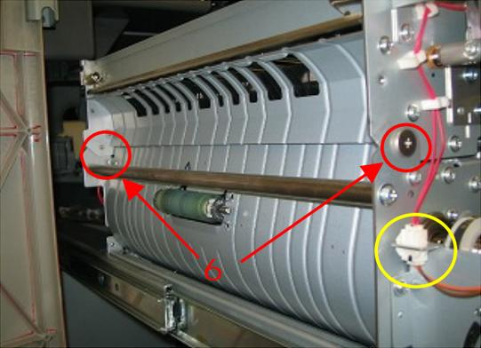
7. Remove the cover and ADU arm (4 screws and 6 connectors)
