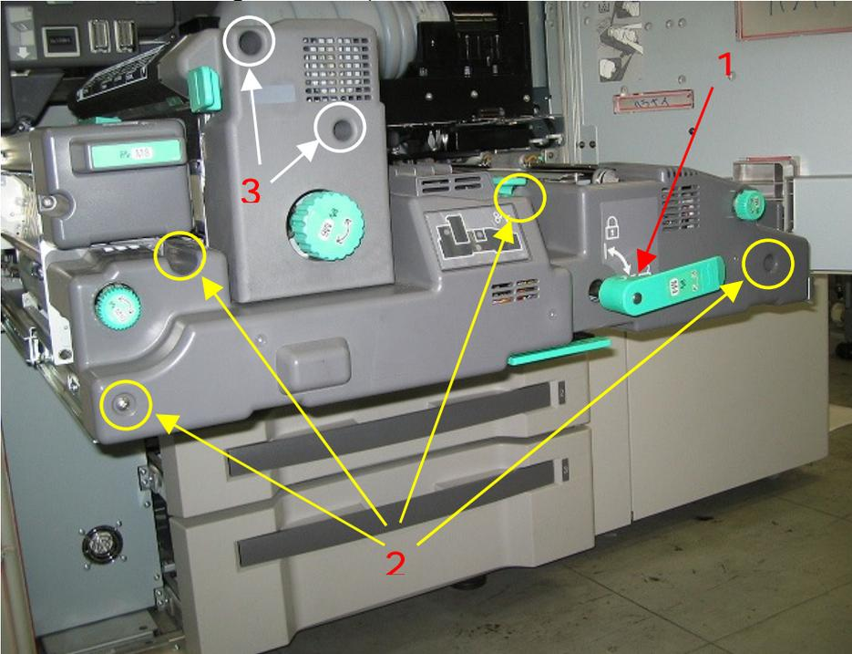
4. Remove the Fusing unit (2 screws)
