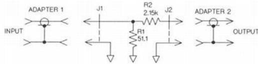
**FIGURE 5-1. IMPEDANCE MATCHING NETWORK SCHEMATIC**
