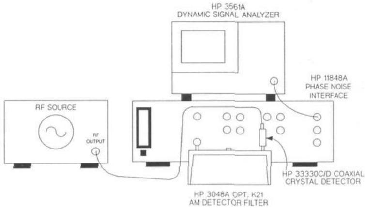
FIGURE 2-1. SETUP FOR AM NOISE MEASUREMENT WITH HP 3048A
