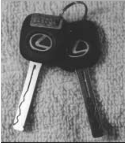
2. The Lexus 4-Track Internal High Security key.
