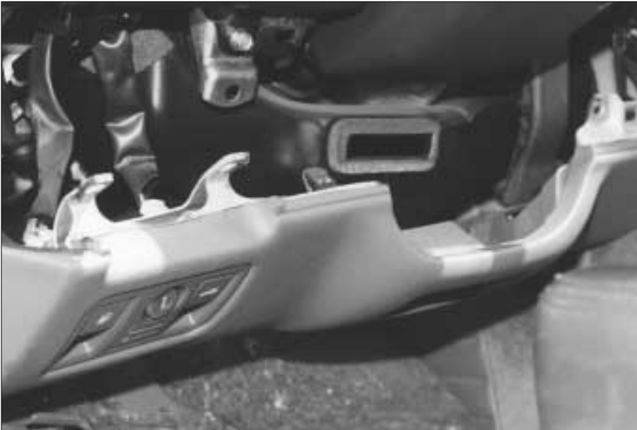
15. The panel lowered.
