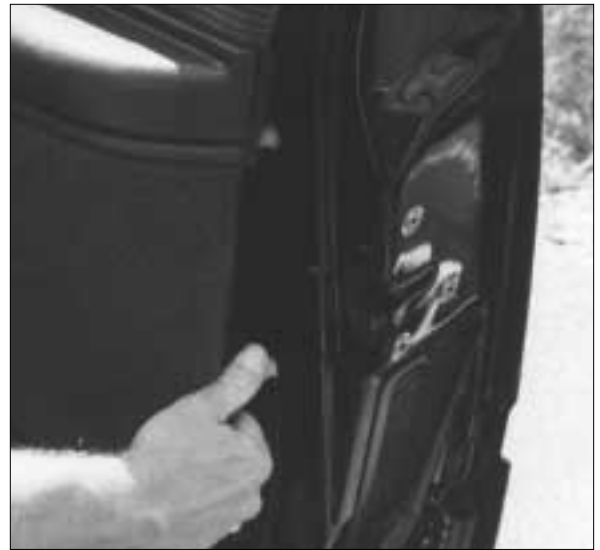
10. Remove the window crank and inner door panel.
