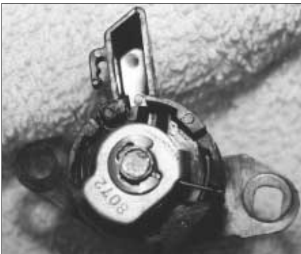
19. Remove the E-clip to remove the tailpiece.
