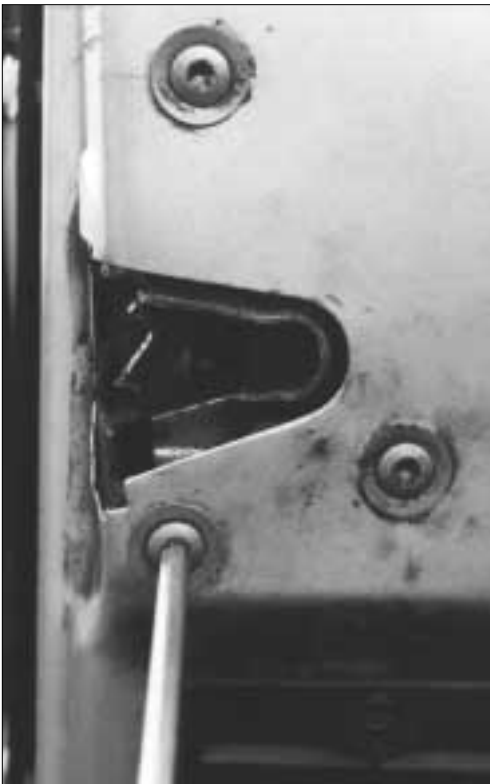
7. Loosen the latch using a T30 Torx screw driver.
