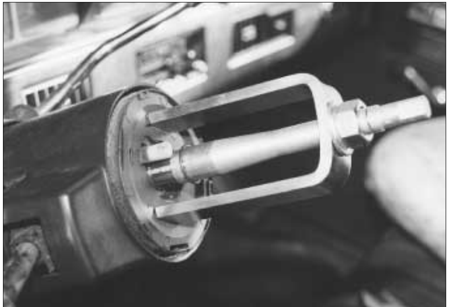
1. HPC's SWLPC-1 Steering Wheel Lock Plate Compressor allows for easy removal and replacement of the steering lock plate retaining ring.
