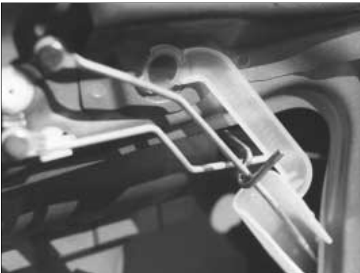
2. Finding the open spot of lock linkage is tricky but not impossible.
