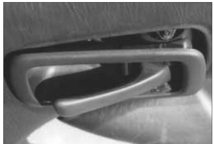
10. Start by removing the door latch release trim. Gently remove the bottom side first and then the top. This part breaks easily.
