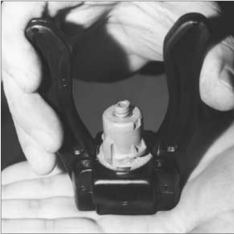
2. The Pro-Lok "Clincher" makes fast, easy face cap replacement.
