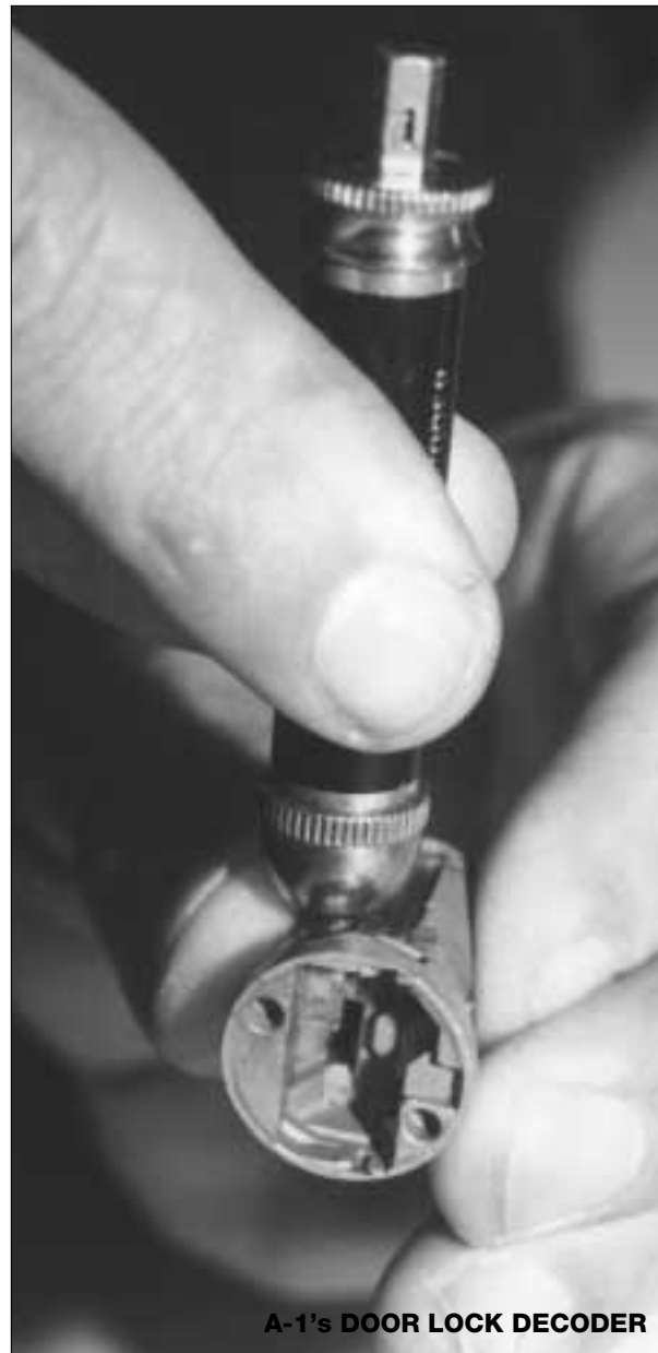
3. Decoders like HPC's GMTD 5 and A-1's GM Door Lock Decoder can help the beginner learn to read GM door locks.
