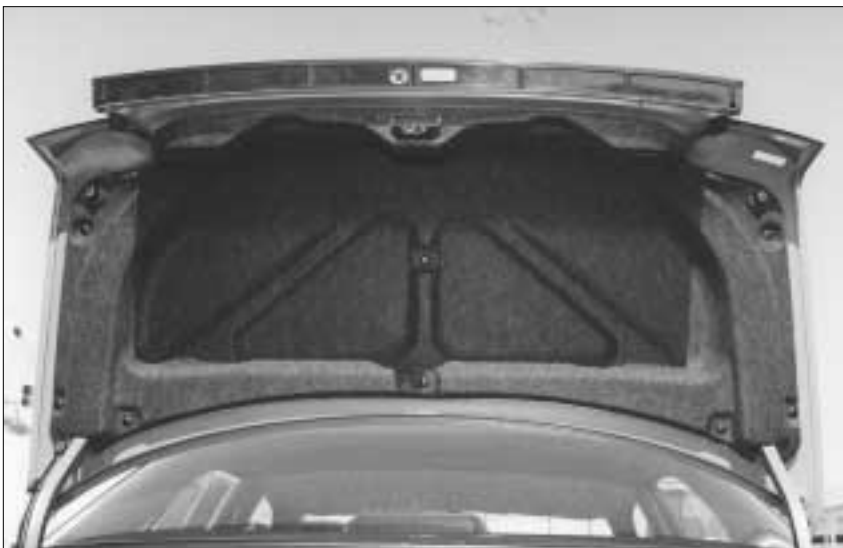
16. This liner must be removed from the deck lid before gaining access to the light assembly and trunk lock.
