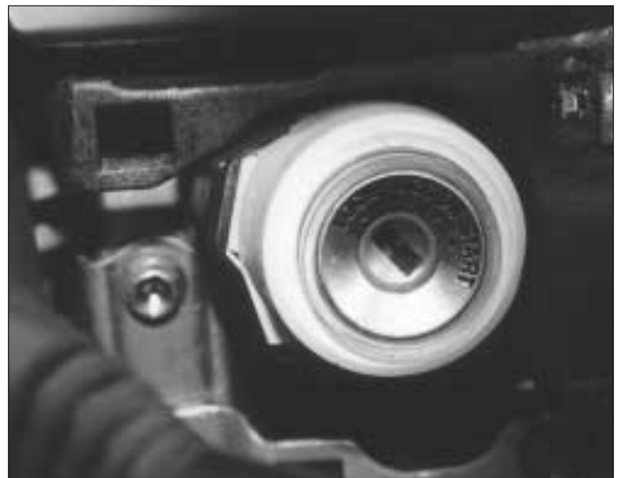
4. Remove the dash cover and the plastic bezel from around the lock.
