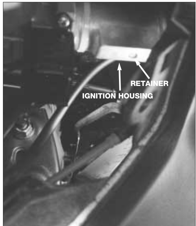
4. The ignition housing is clearly seen from under the dash area. But, it is not necessary to remove the cylinder from this position.
