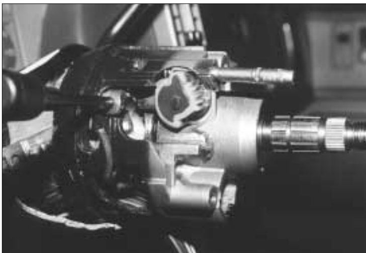
3. Despite the damage to the lower bowl, the sector gear and steering wheel lock bolt remain unscathed.
