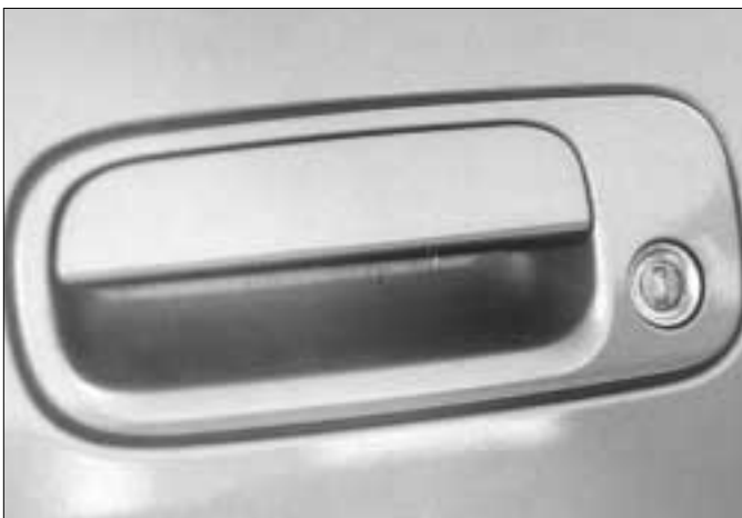
9. The door lock is integrated into the handle.
