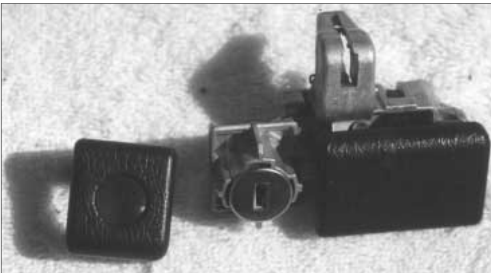
20. Gently remove the plastic cover over the plug.
