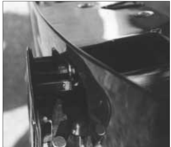
8. Pulling the handle out gains access to the linkage on the door handle assembly.
