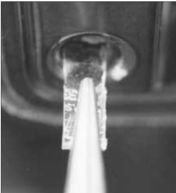
18. After the handle has been placed back into the door, use the special key and pull the lock into its seated position.
