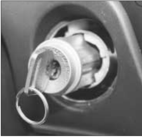
5. Use an L-shaped probe to reach the cylinder retaining button and remove the ignition cylinder from the housing.
