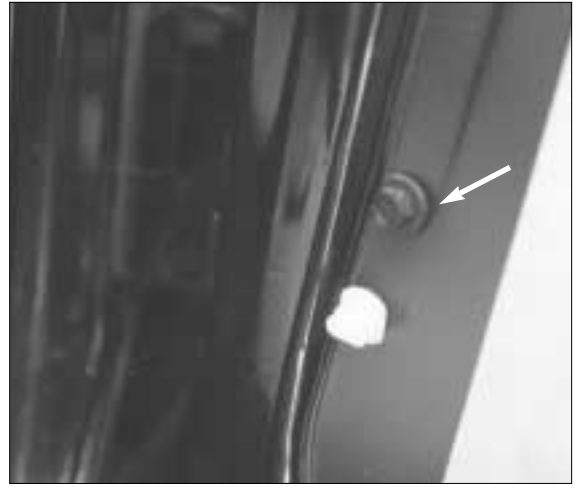
6. Loosen but do not remove this bolt on the inner door panel.
