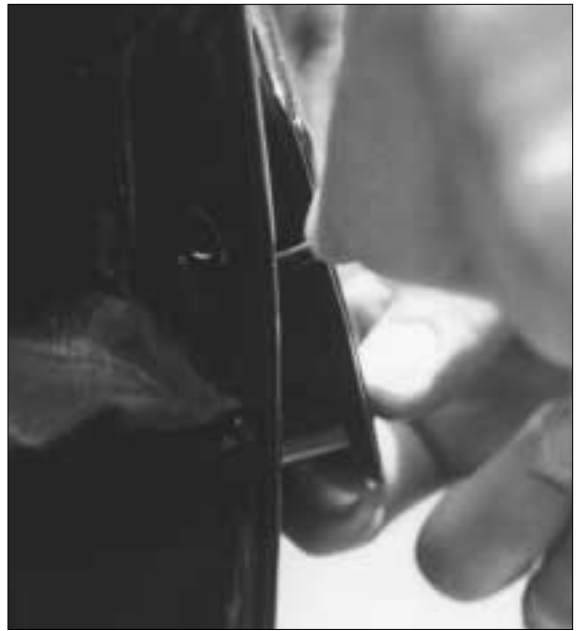
14. Pull the handle out just enough to reach inside with a probe.
