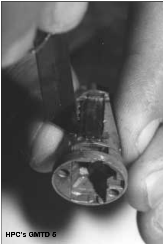
3. Decoders like HPC's GMTD 5 and A-1's GM Door Lock Decoder can help the beginner learn to read GM door locks.
