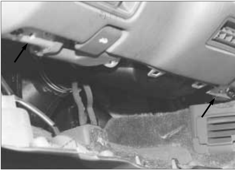
14. The six 10mm bolts needed to lower this panel are easily located and removed.
