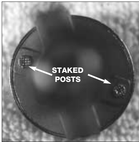
7. The face cap is held to the lock body by both a roll pin and two staked posts.
