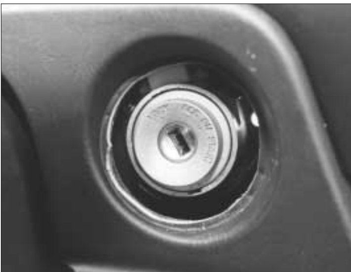
3. Lock with rubber ring and plastic bezel removed.
