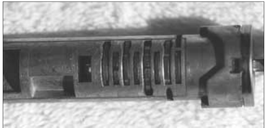
8. These vehicles utilize the Toyota split wafer system.
