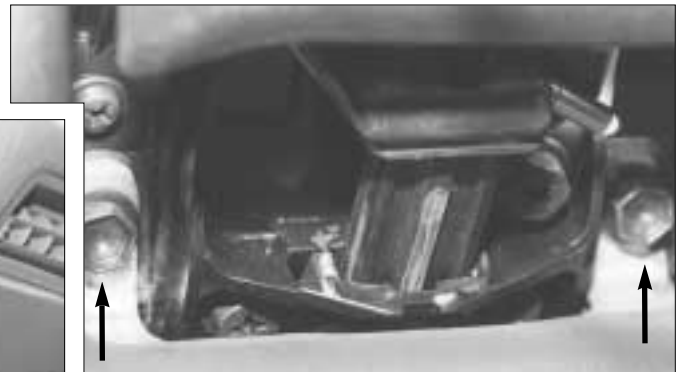
13. Remove three screws and drop the knee bolster or lower panel to get to the trunk release lock.
