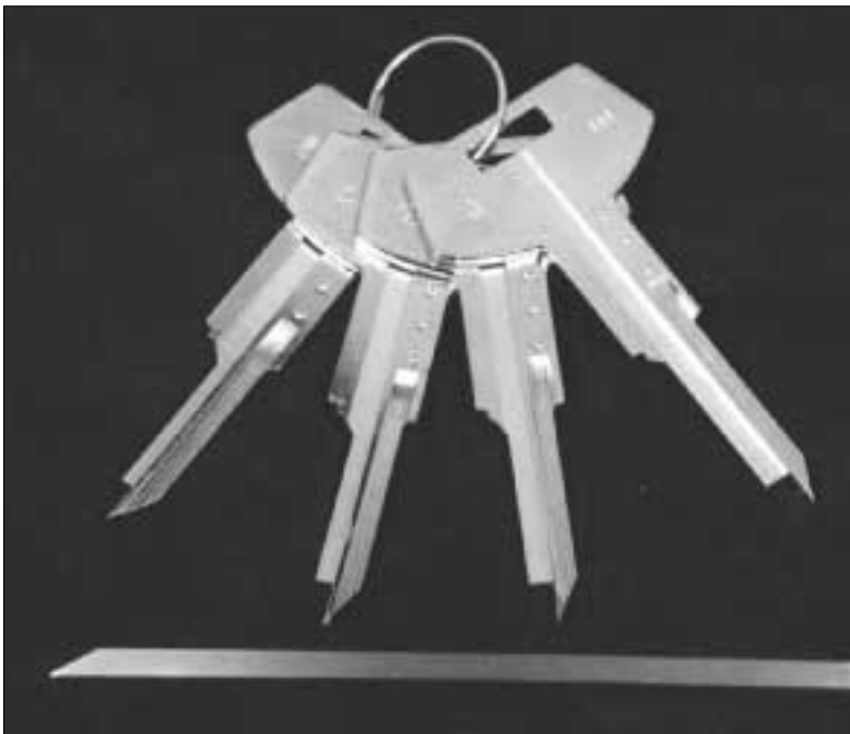
3. Saber Tool's AlphaCracker let's the locksmith generate Alpha Tech keys without disassembly.
