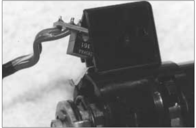
18. Remove the micro-switch attached to the lock.
