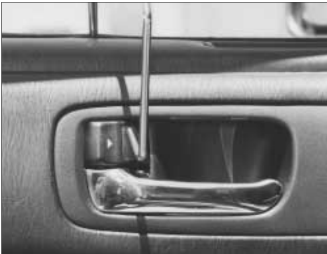
3. Opening the LS400 using an Under-The-Window tool.
