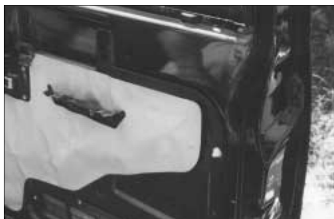
4. The inner steel panel, while needing to be removed, has all the internal door and window components attached to it.
