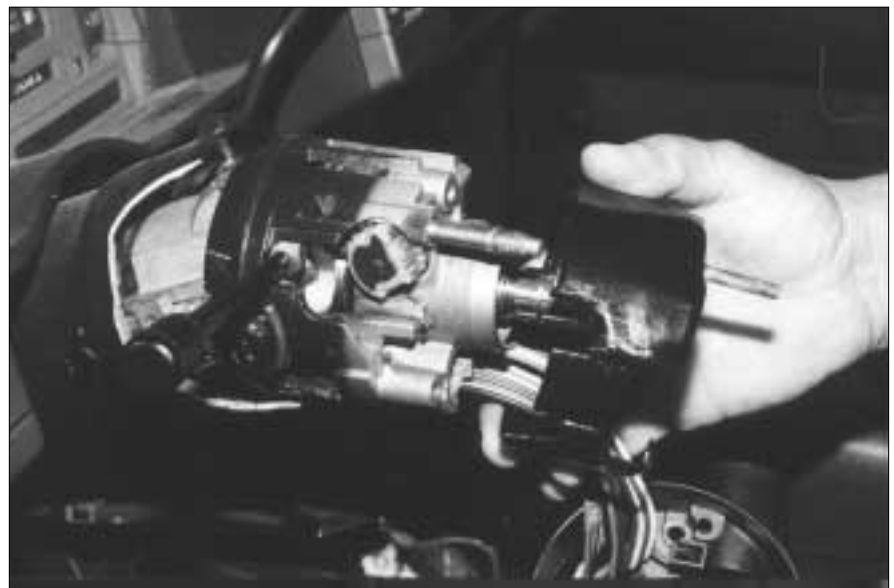
2. An attempt to steel this vehicle resulted in the lower shifter bowl and rack being broken. The steel armored sleeve, however, protected the sector gear and steering wheel lock bolt from attack.
