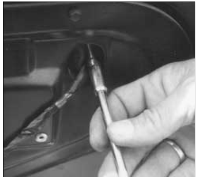
12 Remove the handle retaining screws with a 10mm socket.
