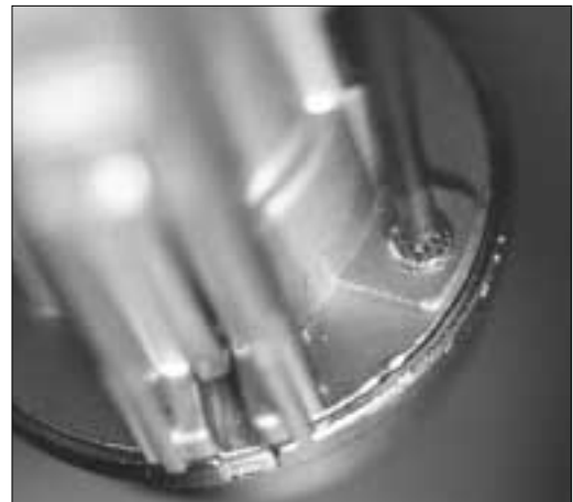
8. Drill a small hole next to the pin and pry it out with a pin punch or scratch awl. Then use a punch and gently tap the staked posts through the body to remove the face cap.
