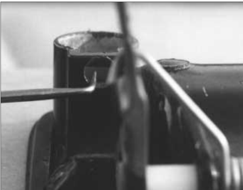
15. Use the probe to depress the lock's retainer and remove it from the handle. The position of the retainer's access hole in the handle and the lock's retainer seen above.
