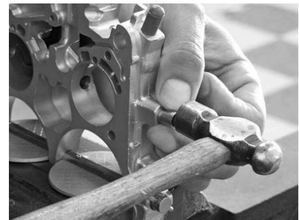
After you've drilled out the throttle shaft hole, gently tap in the new bushing.
