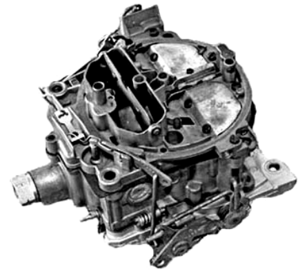
The Rochester 4M carburetor 1966-1969
