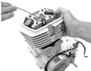
Detach two dowel pins in advance and keep them for re-use.
