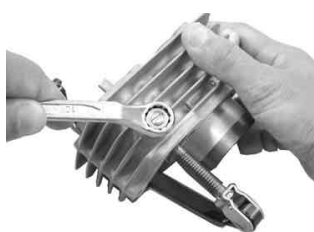
Remove a lock nut and an adjust bolt from the cylinder.
