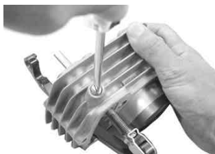
With a cutter or a scraper, get rid of the gasket scraps remaining on the cylinder head plane on which to fit a manifold.
