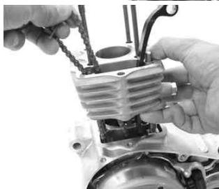
Take off two dowel pins in advance and keep them for reuse.
