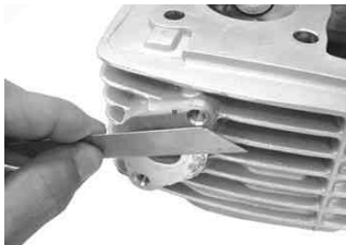
With a cutter or a scraper, get rid of the gasket scraps remaining on the cylinder head plane on which to fit a manifold.
