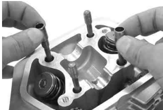
Remove the cylinder head.
