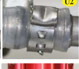
27. Place the small lock ring on the end of a nut-driver or socket with its flared end inwards towards the socket as shown in figure 'U1'.
