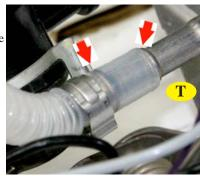
25. Slide the crimp clamp over the flex fuel line and position it between the two bumps on the metal fuel feed-line as shown in figure 'T'. Using a pair of side cutters or fence pliers crimp the clamp as shown in figure 'U1' and 'U2'. **Do not use excessive** force which may cut through the crimp clamp.
