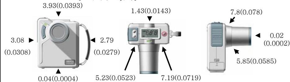
Leakage radiation at 1cm from case surface is less than 8mR/h(0.08mGy/h).
