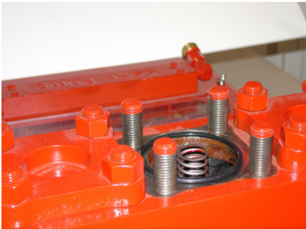
16.) Install the discharge spring.
