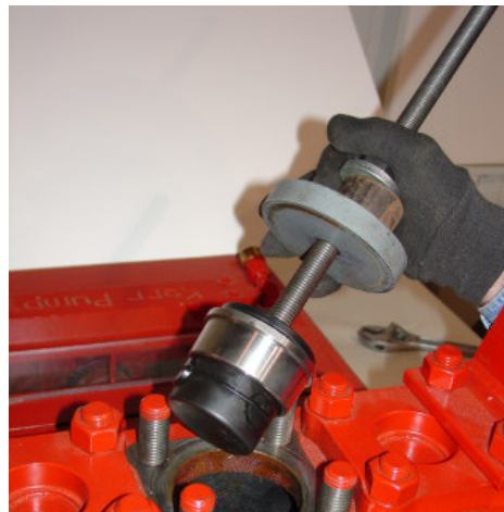
11.) Remove the puller assembly with seat attached.
