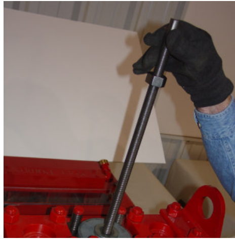
8.) Turn the puller rod until the pins are fully extended.
