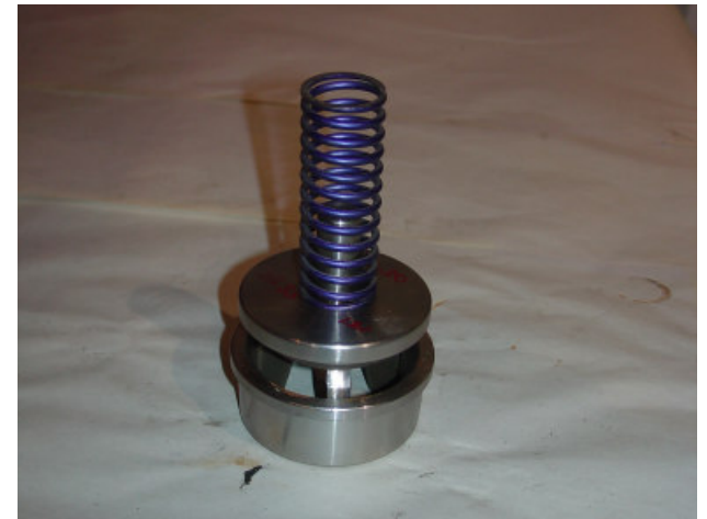
15.) Install the suction spring.
