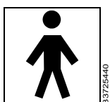
Figure 8.1 Type B ‘applied part’ symbol
