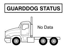
• If the engine is started to soon for the system to complete a proper engine level reading the following screen displays.
