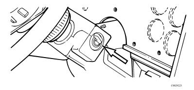
This switch starts the engine (turn the switch clockwise) and activates the accessory relay (turn the switch counterclockwise). When the switch is turned ON (in a clockwise direction), a warning buzzer sounds if air system pressure is below  $448 \pm 34$  kPa  $(65 \pm 5 \text{ psi})$  or if there is low oil pressure. The buzzer shuts off as soon as sufficient air/oil pressure is restored.
