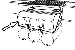
The CXU vehicle has two styles of battery boxes available. One is covered with a plastic cover, the other cover is polished aluminum.
