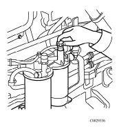
2. Pump the hand primer until the force of pumping increases.
