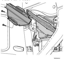
To provide comfortable and clean fresh air in the cab, the heating and air conditioning system is designed with a replaceable filter.
