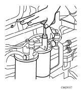
**Note:** When the fuel system is empty, 200 or more pump strokes may be needed to properly prime the system.
