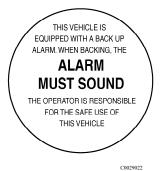
A POLLAK BACK-UP ALARM HAS BEEN INSTALLED ON THIS VEHICLE. MAKE SURE IT IS IN WORKING ORDER BEFORE OPERATING VEHICLE.
