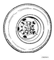
Look for cracks around the hand hole, stud hole and wheel. Look for broken studs, wheel damage or improperly seated lock rings.
