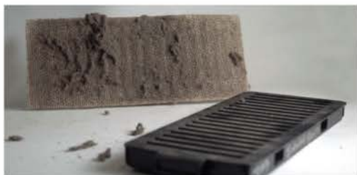
3M™ HAF-E filter after three months use in typical casino setting.
