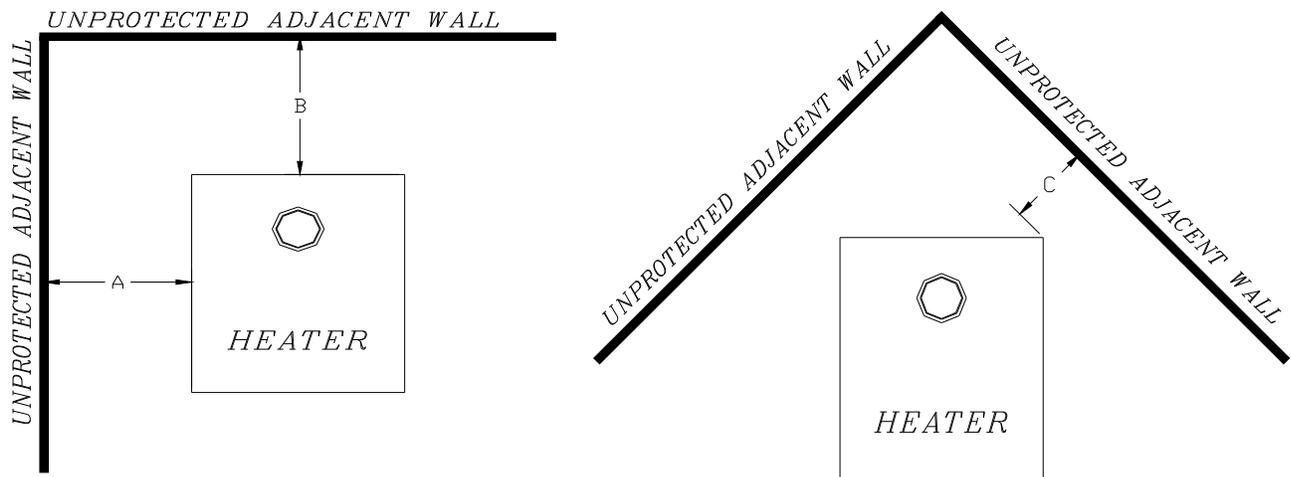
**FIGURE 1.3 Clearances to combustible materials**
